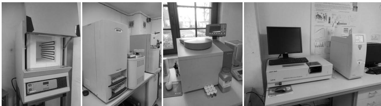
Figure 2. The lab equipment used in presented researches (from the left: muffle furnace; atomic absorption spectrometer – AAS - dedicated to the determination of carbon, hydrogen, nitrogen and sulphur content in solid materials; calorimeter bomb; AAS dedicated to the determination of mercury content in solid materials; ion chromatograph).
