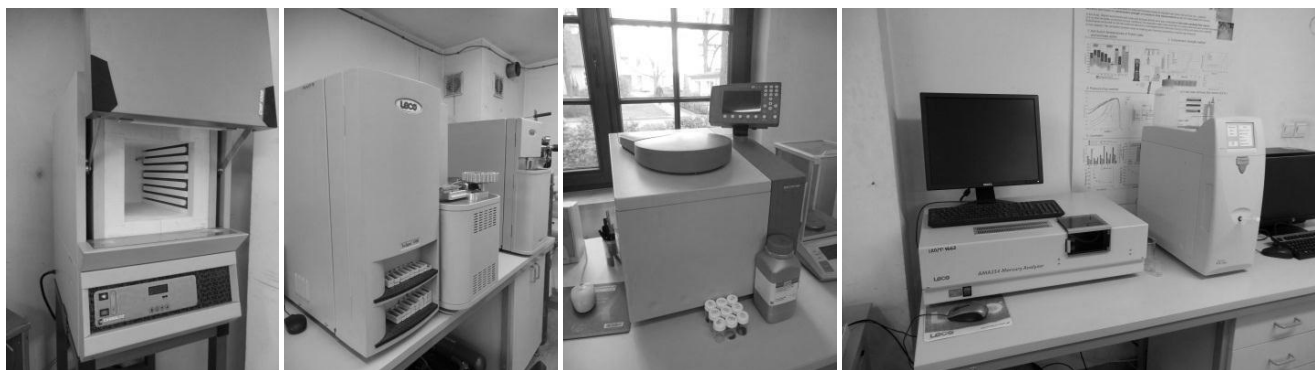
Figure 2. The lab equipment used in presented researches (from the left: muffle furnace; atomic absorption spectrometer – AAS - dedicated to the determination of carbon, hydrogen, nitrogen and sulphur content in solid materials; calorimeter bomb; AAS dedicated to the determination of mercury content in solid materials; ion chromatograph).
