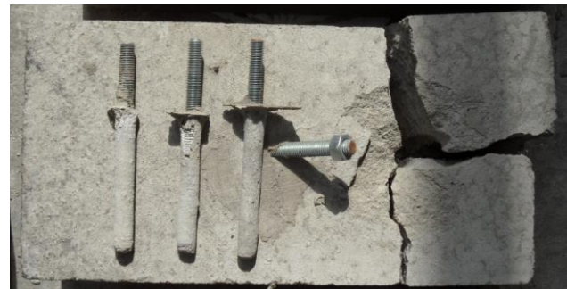
Fig. 11. Drawn anchors after the pull-out test.
