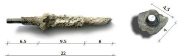
Fig. 7. A view of destruction fixing anchor with concrete substrate.
