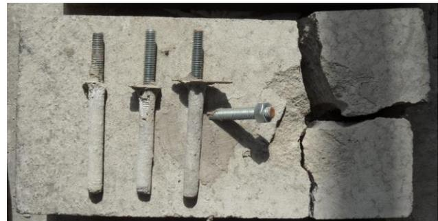
Fig. 11. Drawn anchors after the pull-out test.
